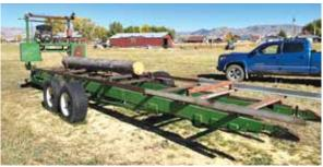
Refurbished sawmill mounted to a bale frame is 25 ft. long.
