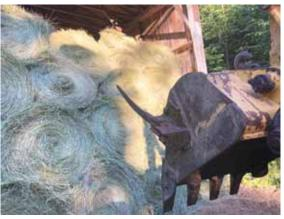
Merkley reinforced the bucket with steel plate, then attached the bale spear.
