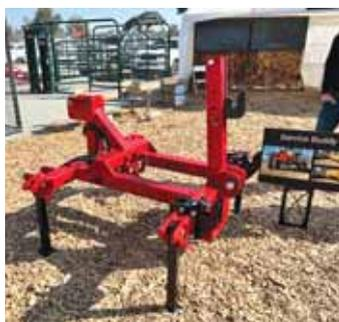
**Service Buddy makes the bottom of implements accessible from the rear and can lift up to 6,000 lbs.**
