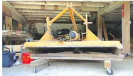
Rolling mower carrier allows for easy storage and retrieval.
