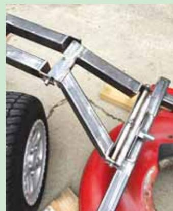
Each walk-behind mower deck got its own frame bolted to it. These frames hinge to the main frame, providing articulation up and down.
