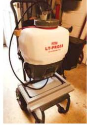
Backpack sprayer is mounted to an old pressure washer frame.
