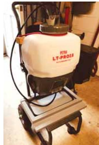
Backpack sprayer is mounted to an old pressure washer frame.
