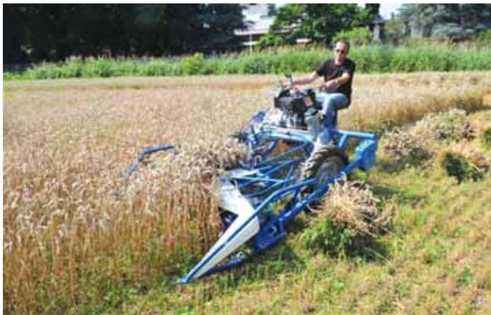
BCS 622 reaper binder has a working width of 55 in. and is available as a motorized cutting bar without binder.
