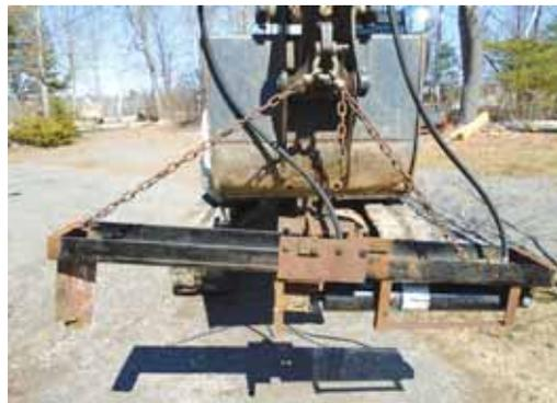
Jim Schoonhoven used pieces from an old truck frame to build this "upside down" wood splitter that attaches to his Bobcat excavator.
