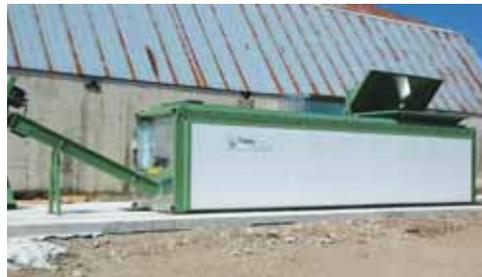
"Our BioRoter, combined with a biomass-fueled furnace or boiler, can create a biosecure, closed-loop on the farm," says Wiebe. "Load it up in the morning, and 24 hrs. later you can unload material with 10 to 15 percent moisture, ready to be burned with wood chips or other biomass."
