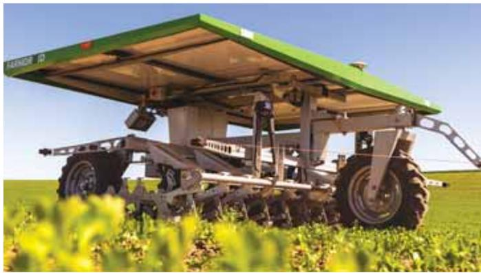
**Each robot weighs less than 1,800 lbs. and can cover as much as 13 acres per day. It has a working width of just under 10 ft. and can be configured to place seeds in 4, 6 or 8 rows.**
