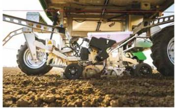
Seeding units can do single or multiple in-line seed placements. An infrared sensor detects each seed drop and notifies the onboard computer if one is missed.
