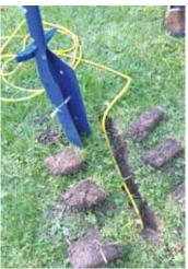
Trenching tool digs a 2 1/4-in. trench at adjustable depths with minimal damage to lawns.
