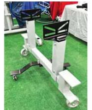
Peters designed the splitter stand to work with tractors large and small by simply replacing the support legs. A short set works with smaller and utility tractors. A longer set fits bigger row crop tractors.
