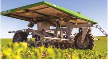
Each robot weighs less than 1,800 lbs. and can cover as much as 13 acres per day. It has a working width of just under 10 ft. and can be configured to place seeds in 4, 6 or 8 rows.
