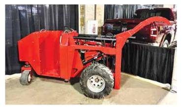
Front-drive wheels with their 47-in. width can telescope out to a 63-in. wheelbase for greater stability.
