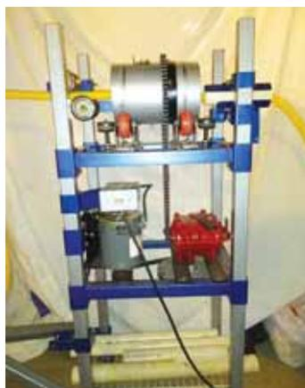
**Bennett made a machine to custom cut PEX tubing for use as protective hose wrap.**
