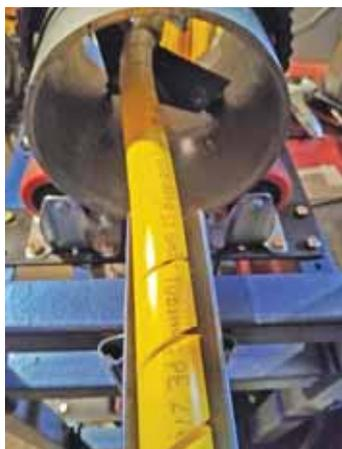
**Hose wrap cutter shaving PEX exiting the cutter.**
