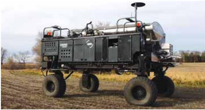
Autonomous platform is equipped with front, rear or 4-WD steering. It can be driven forward, backward or sideways.
