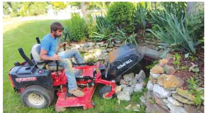
"I welded a bracket on the front of the mower for the wheelbarrow to hinge off the mower. It's easy to dump by hitting reverse really fast," Stokely says.
