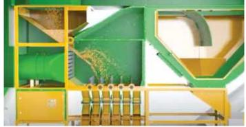
Metra grain cleaners range from 200 to 8,000-bu/hr. capacity and have a cleaning chamber sized for optimum air and seed flow.
