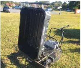
Flock Buddy can fit through standard 36-in. doors, allowing it to move easily from one poultry house to another. With a battery that lasts up to 8 hours, it's built to withstand harsh
