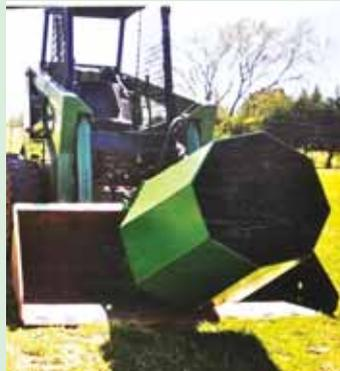
Tumbler drum was once used for polishing ball bearings.
