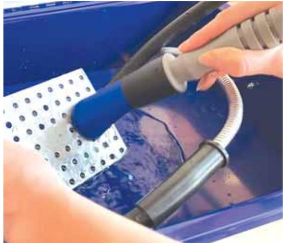
**Flow-Thru cleaning brushes connect to a hose or parts washer and come with poly or brass bristles.**
