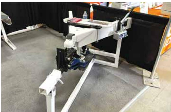
**A WD system is needed if a trailer's gross tow weight is more than 50 percent of the vehicle weight, if the tow vehicle sags when hooked to the trailer, and if it's difficult to steer or stop.**
