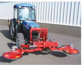
Doublebladed mower attachment can be mounted on both sides of tractor using existing hydraulics to save time by mowing both sides in orchards.
