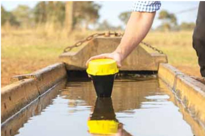
If the tank goes dry for some reason, the accelerometer sensor sends a message when the Water Rat tilts 30 degrees through a SIM card. It also sends two messages daily that all is well.
