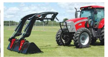
Operator drives into the arms for an automatic auto-lock connection with no tools or pins required.
