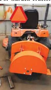
Evan Waa used his laser cutter to make body pieces for his shop-built stump grinder from an old welding table damaged in a fire. Waa says the laser does an excellent job of minimizing waste while cutting different size pieces from a large sheet of steel.
