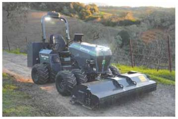
TeleFarmer targets pre- and post-harvest tasks such as weeding, spraying, mowing and transporting with their manual, remote-control or autonomous modes of function.
