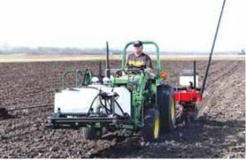
Hubscher attached the planter modules to a 3-pt. toolbar on his compact Deere tractor. He fabricated a skid frame of 2 by 2-in. steel tubing with pockets for forks mounted on his Deere loader.
