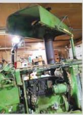
Bunniss hood remover is articulated in four directions, swivels, and will stay where he sets it, making it possible to place the hood back on the tractor, level on all planes. It's fully adjustable and can be used for large and small tractors.
