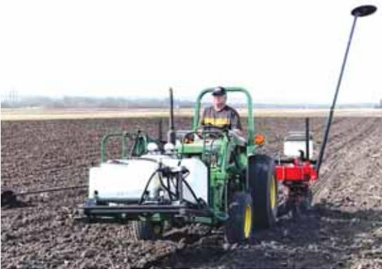
Hubscher attached the planter modules to a 3-pt. toolbar on his compact Deere tractor. He fabricated a skid frame of 2 by 2-in. steel tubing with pockets for forks mounted on his Deere loader.
