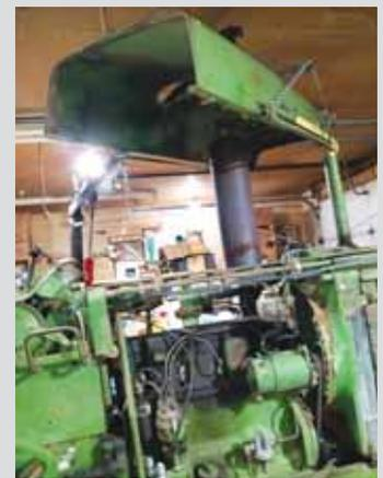
Bunniss hood remover is articulated in four directions, swivels, and will stay where he sets it, making it possible to place the hood back on the tractor, level on all planes. It's fully adjustable and can be used for large and small tractors.
