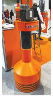
A combination of pedestals and grain cooling fans cool crops quickly to prevent insects, conserve quality, reduce waste, and meet crop assurance requirements.
