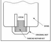
Carburetor repair kit allows for rebuild the stem bottom, saving the expense of buying a replacement.
