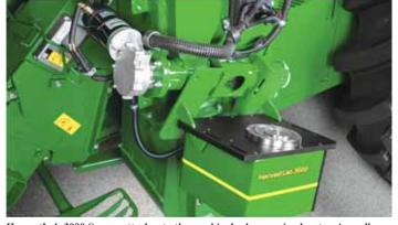
HarvestLab 3000 Sensor attaches to the combine's clean grain elevator. A small motor drives an auger that pushes grain past the near-infrared sensor as the combine is harvesting.
