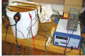
Electroplating tank and power source.
