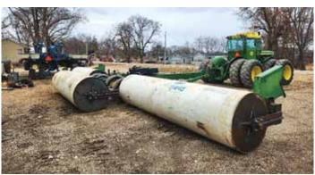
Farmer built a three-section 42-ft. wide field roller using the frame and wheels from a Deere 7000 16-row planter and three used anhydrous tanks.
