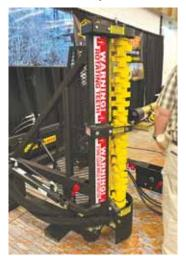
Weighing only 265 lbs., the 48-in. Baby Beaver cuts through limbs and trees up to 3 in. in diameter at 4.500 rpm's.
