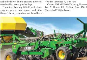
Installation involves the removal of the factory-installed gauge wheels and beams from the frame. Once the TerrainFlex walking beam has been installed and the gauge wheels added, the air drill is ready to go.
