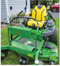
Fox made a grab bar for his mower using 3/4-in. steel pipe.
