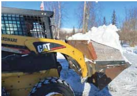
"It more than doubles the capacity of the (1/2 cu. yd.) bucket." Tucker says, for light loads such as snow, sawdust, and wood shavings. "And by using the mesh, I can easily see through it for driving and loading and safely look over or under it when it's loaded."
