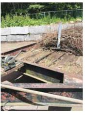
The rope pulls an L-shaped metal bracket to the back of the trailer. As he loads the trailer, he packs the brush around the upright bracket.
