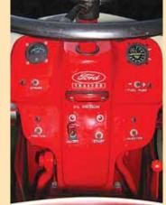
Dash has switches to operate the jet turbine.
