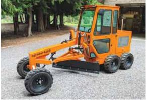
"I ended up using Toro zero-turn lawn mower individual trans-axles so I could spread the frame a bit and made some linkage to tie the two drive motors together," Hadler says.
