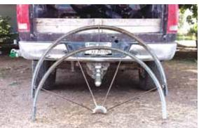
Half-section of spare wheel bolted on outside of wheel acts as a cam to lift wheel line irrigator.
