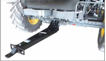
NDY makes a bolt-on hitch for combines to tow a wagon, blower or spreader.
