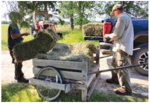
Garden cart made from recycled pallets and bicycle wheels works well and distributes weight evenly for chores
