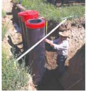
The columns measure 8 ft. in length and are buried in the ground to a depth of just under 7 ft. leaving approximately 20 in. sticking up out of the ground.
