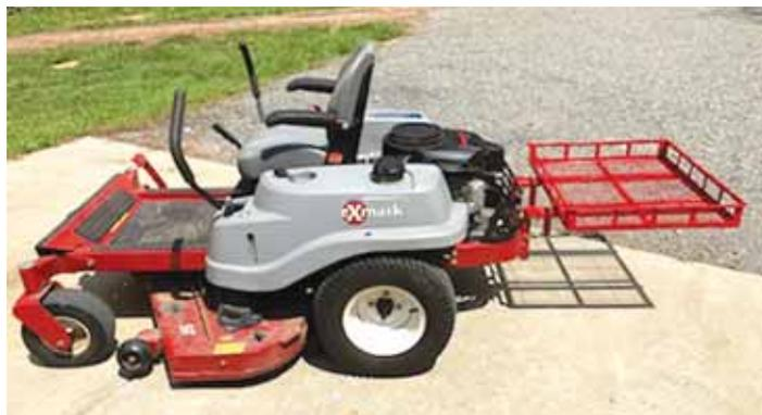
The metal basket is bolted onto a plate attached to the mower. There's 1 1/4-in. square tubing that 1-in. tubing slides down into.
