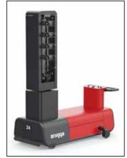
Pollination robot has cameras to determine when to use air pressure to shake pollen loose.
