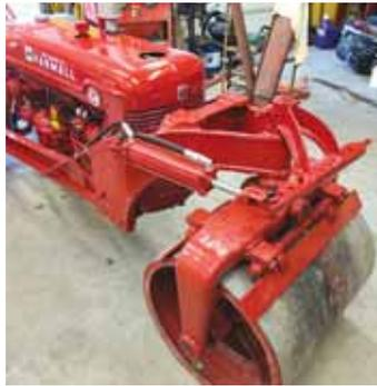
Original worm gear and steering was replaced with a hydraulic cylinder.
