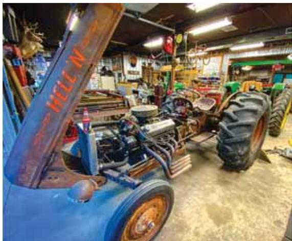
Del Ponte stripped the engine, cooling system, gas tank and steering from his 8N, then extended the chassis and hood to fit the 460 engine. Hot rod headlamps and combine tires add to the look of his custom 8N.
