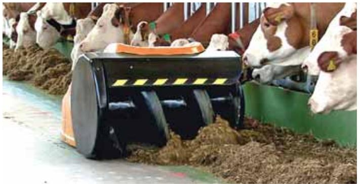
The robot follows a trail of magnets drilled into the concrete floor. The operator can use the touch screen on the robot to control it or use an app-equipped device to program it to operate at different times during the day.
