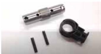
Kits from Bryant Combine Parts repair worn reel pipes. The bearing and holder are removed, the worn pipe is cut and the section slides into the OEM pipe, and is pinned in place.
