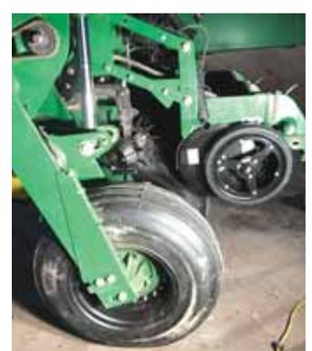
Aircraft tires last longer than OEM implement tires because they are thicker and made for heavier loads.
