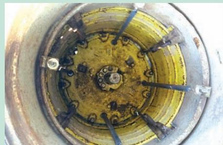
These two plates are used to mount the big flotation tires up front. Forde used a truck rim to make a "triple clamp" with welded-on bracing.
