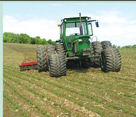
Forde cultivates newly emerged crop at a 45 degree angle using a rotary hoe with the hoe wheels turned backward.
