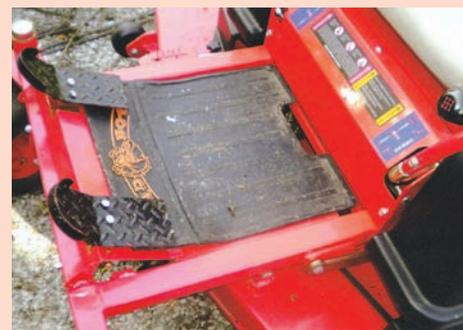
Pushing on toe portion of foot pedal controls forward movement, and pushing down on heel portion controls reverse. Pushing down farther either way controls speed.
