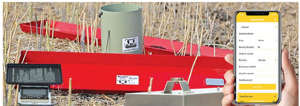
**Drop pan attaches magnetically under combine and is dropped remotely while harvesting to collect a sample of chaff and straw. A downloadable app shows bu. per acre grain loss.**
