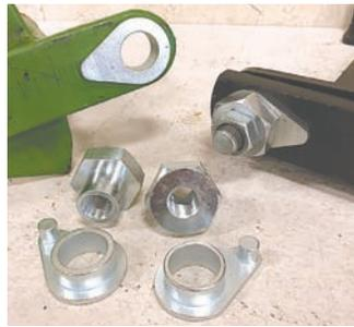
Flange bushing has a small built-in “dowel”.
