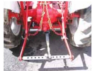
Mike Wingler uses the 3-pt. hitch on his tractor to lift front-mounted implements, with help from a subframe, scissors lift, and boom arms.
