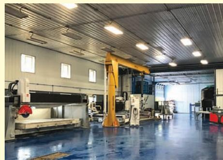
Jeff Hoeft converted his farm shop to build customized countertops out of stone slabs, using an Italian-made computerized CNC saw to cut the stone.
